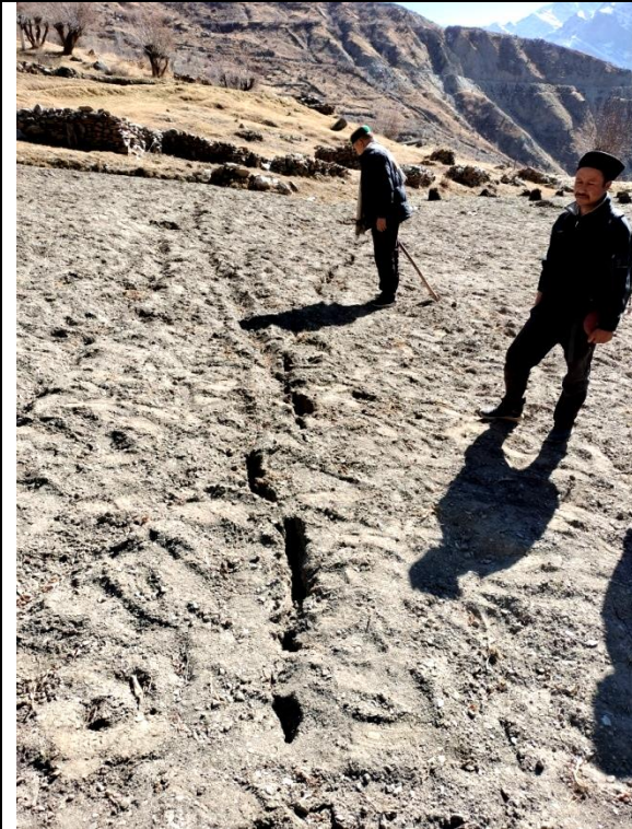
Fig. 8: NNE-SSW trending transverse cracks observed in agricultural fields near the periphery of the active slide 2.
